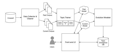
Figure 1: The architecture of the tool.
