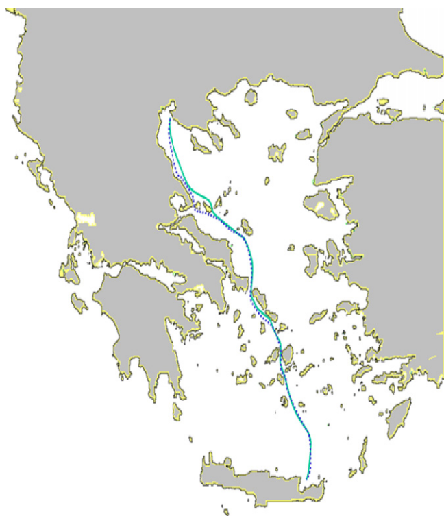
Fig. 6. Optimal route calculated from the port of Thessaloniki to A. Nikolaos for the case shown in Fig. 5 with the proposed algorithm (solid line) and with the application of genetic algorithms (dashed line).
